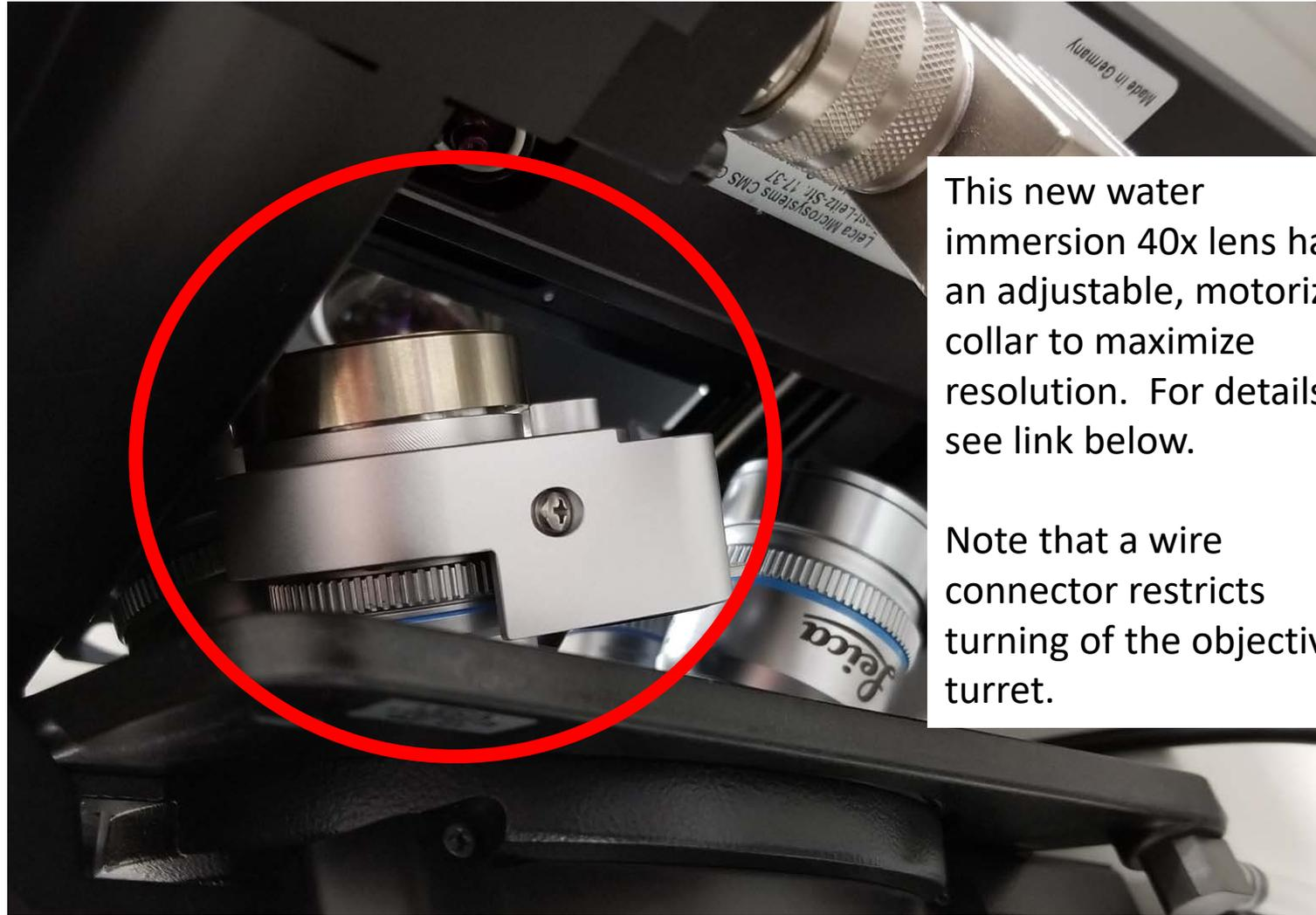
This new water immersion 40x lens has an adjustable, motorized collar to maximize resolution. For details, see link below.
